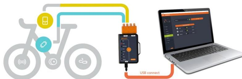
Fig. 1-1 Hardware connection
